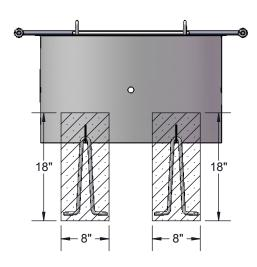
Attach the ground staples to the Fire Ring before inserting then into the concrete footings.
