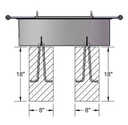
Attach the ground staples to the Fire Ring before inserting then into the concrete footings.
